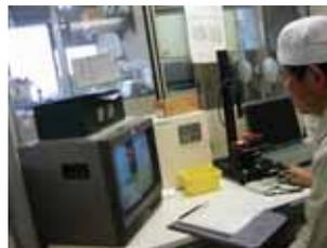
After completion of needlepoint operation, in-process inspections are performed, with each production lot as a unit, thus severely checking needle lengths in terms of accuracy requirements. Then needles flow to the cleaning process, which is the next one.
