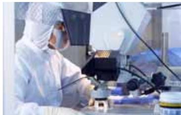
A magnifying microscope is used to carefully check the needlepoint condition, with each production lot as a unit.
