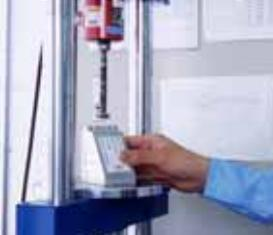
Items such as the needlepoint condition, the adhesion strength of joints between needle shafts and needle tubes, and the drawing tension between needle shafts and needle bodies are subjected to in-process inspections, with each production lot as a unit, thereby achieving the quality suitable for the next process.
