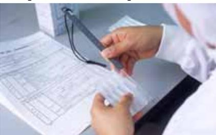
In-process inspections are performed, with each production lot as a unit, to check the indication condition, the sealing condition, etc., thereby providing products with air-tightness capable of steadfastly maintaining product sterility suitable for the sterilization process, which is the next one.
